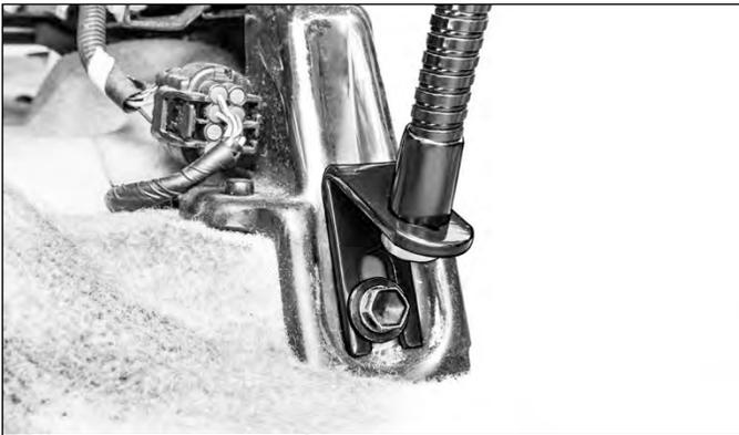
**4** Attach Dual-T-compatible holder or device (not included).
